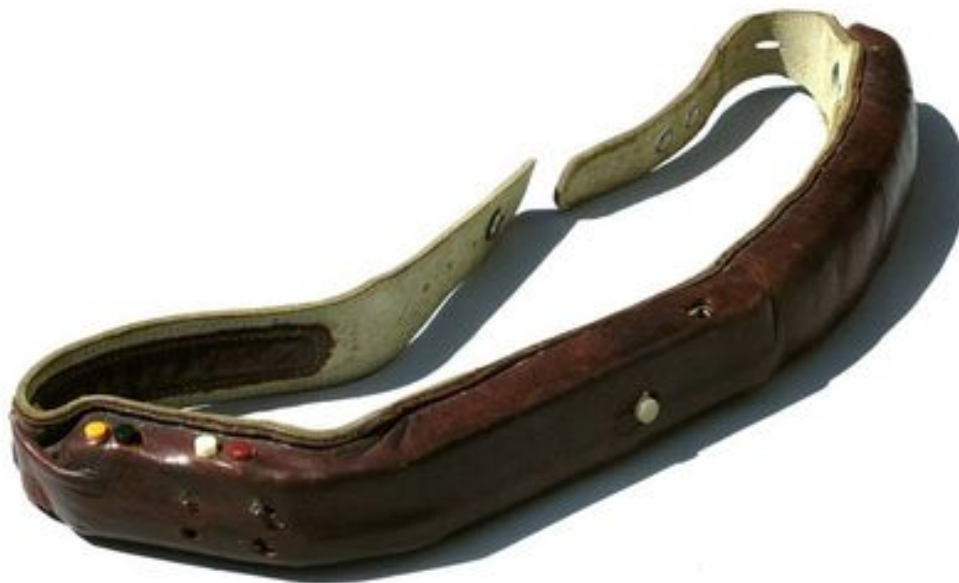
Robert Gable's belt-mounted transceiver, capable of sending and receiving tactile signals. Source: Robert S. Gable
